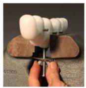
Use the wing nuts to tighten the stake from the bottom side of the vise jaws. This will keep the stake stable in the vise when hammering. Since vises vary in size, the washer supplied with the anticlastic stake may be too large or small. Hardware stores have washers in many sizes. This simple system is easy to use, and it is inexpensive to replace the bolts, washers, or wing nuts at a hardware store if they are lost or damaged.
