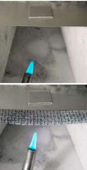
▲ Unsupported, flat pieces of Argentium (top) can sag during soldering; be sure to support the metal (bottom).
