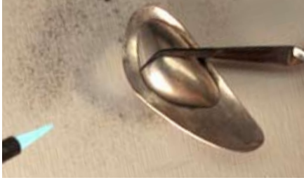
▲ Argentium can be fragile when heated, so it's best to use binding wire to hold the piece in place while soldering (top) rather than using cross-locking tweezers (bottom).
