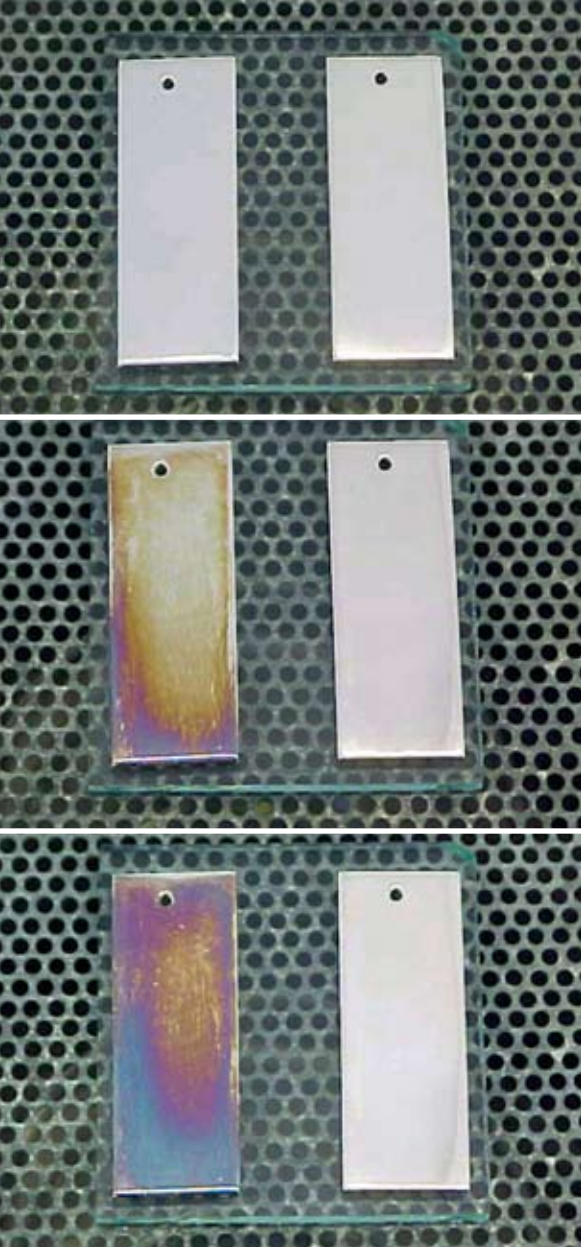
▲ As a tarnish test, samples of traditional sterling silver (left) and Argentium sterling (right) were exposed to a diluted ammonium polysulfide solution and photographed at 30-minute intervals.
