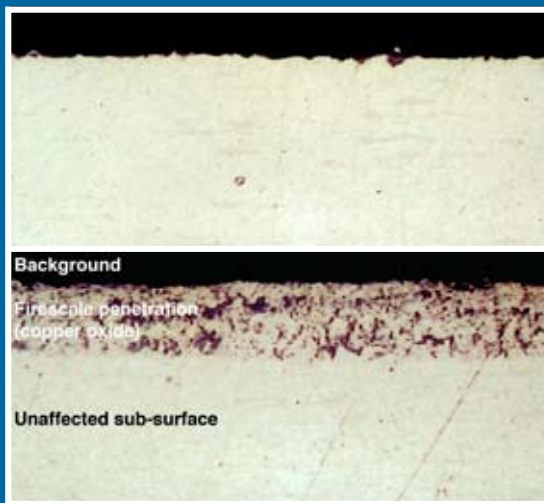
▲ Microscopic cross sections of Argentium (top) and traditional sterling silver (bottom) heated at 1076°F (580°C) for 1 hour show a marked difference in firescale penetration.
